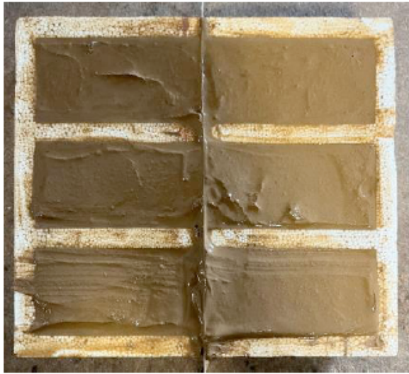
Figure 3: Molds containing the prepared raw earth mixture.
