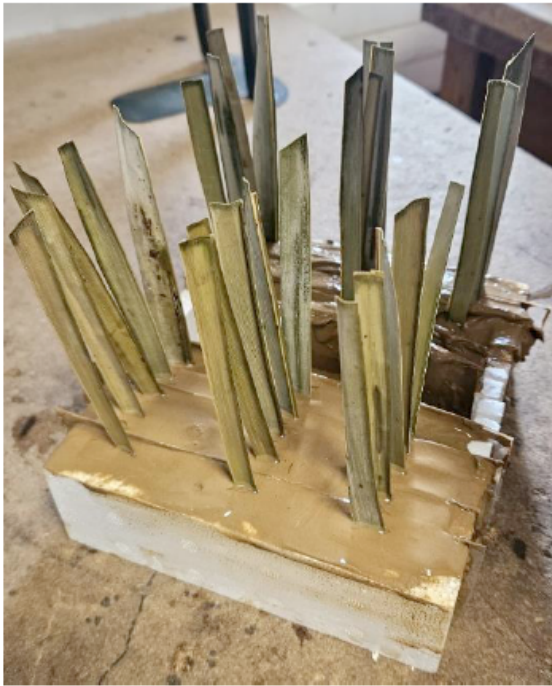
Figure 6: Preparation of specimens for fiber pull-out testing.
