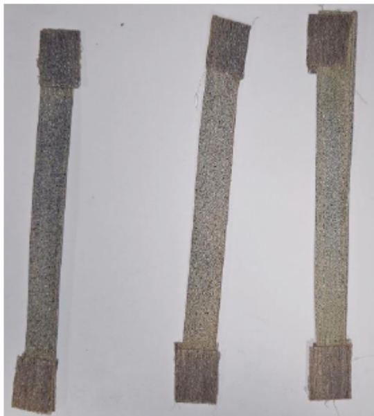
Figure 1: DPF samples with reinforcement at the gripping zone.
